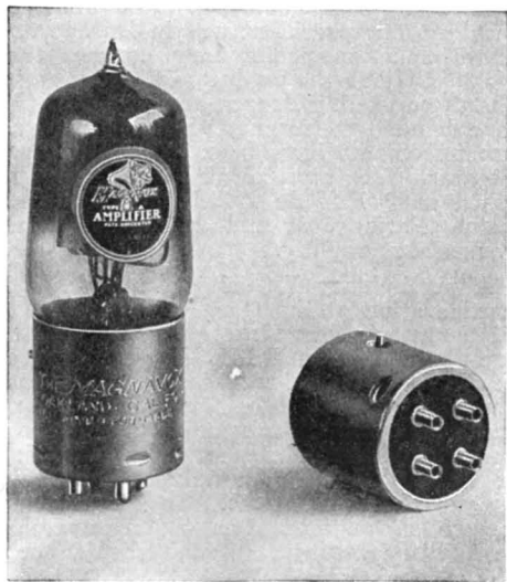
FIG. 4. COMPLETED TUBE AND VIEW OF BASE SHOWING BAKELITE INSULATION.
