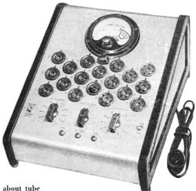
No longer is there any need for worrying about tube checker obsolescence. Again Weston has supplied the solution; providing a design with 18 sockets, 11 of which are wired to test all of the present tubes, some 90 in number. The remaining 7 sockets are spares, and can be quickly wired in to test some fifty-odd additional tubes, when and if these tubes appear on the market.
