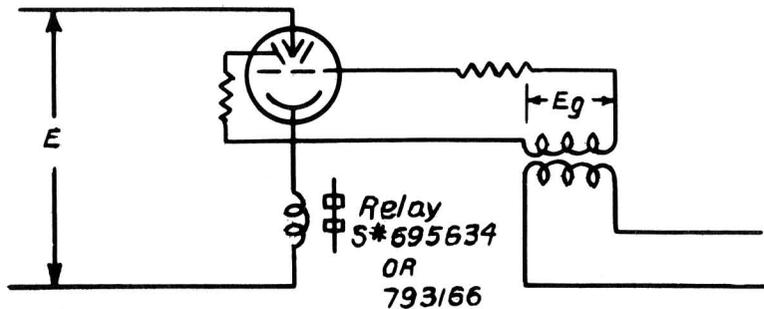
FIG.\*12-EXTERNAL BIAS VOLTAGE CONTROL
