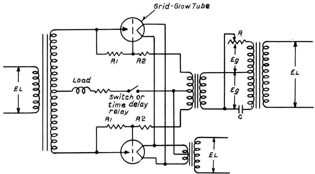
Phase shift control circuit Full wave rectification
