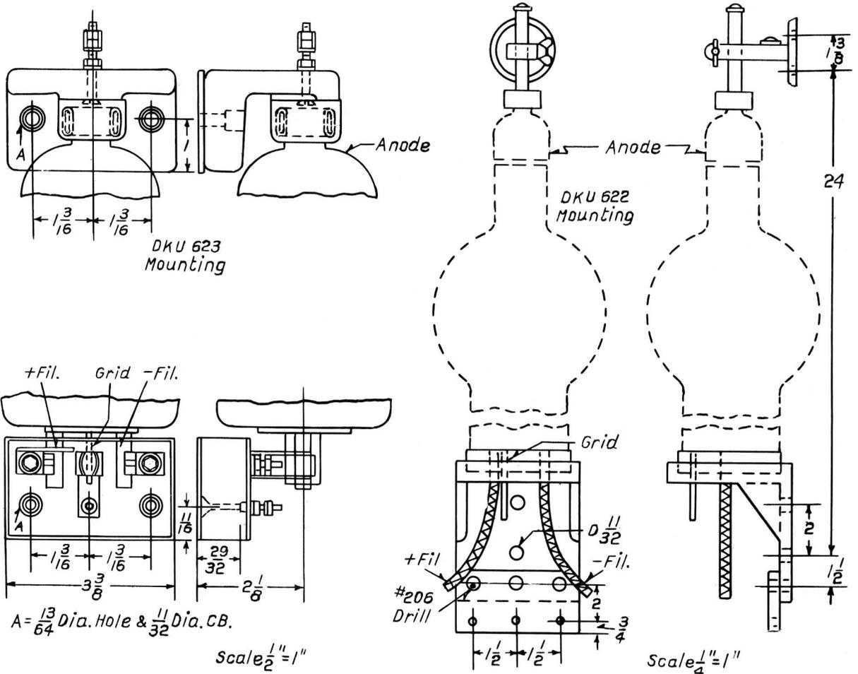
FIG. 2-DIMENSIONS OF TUBE BASES
