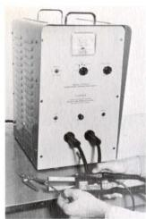
BY SELECTING THE LOW RANGE, 3 WATT-SECONDS CAN BE PRE-CISELY SET AND CONSISTENTLY REPEATED TO WELD A .004" COP-PER-IRON THERMOCOUPLE JUNC-TION WITH A VTA-24 HANDPIECE.
