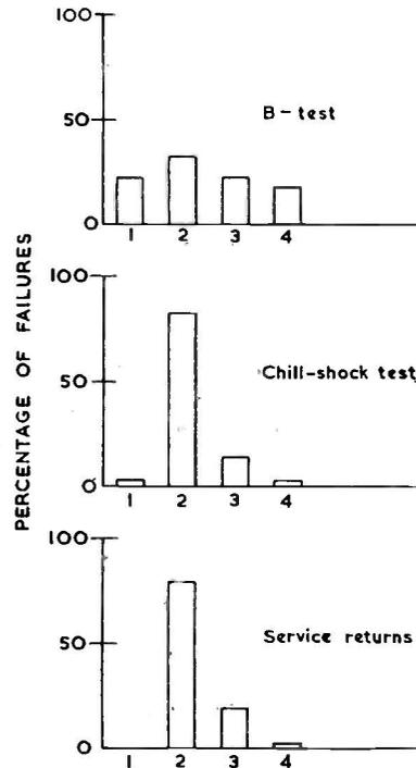
Fig. 4. Fracture type-distribution for 'B' test chill-shock test and service returns
