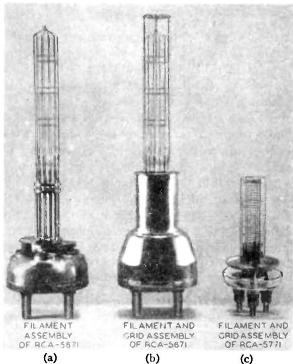
Fig. 1(a-c)—Self-supported, multistrand, thoriated-tungsten filament assemblies (with and without grid assemblies).
