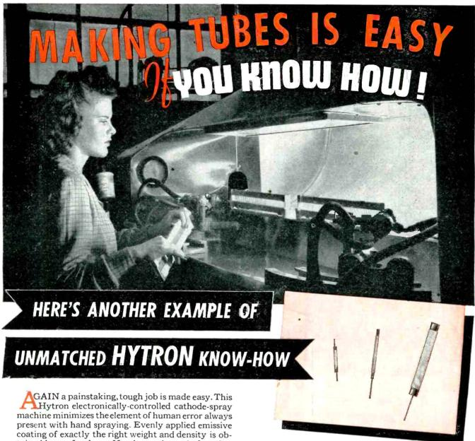
tained hour after hour. Number and speed of coating passes, distance from spray guns to cathode sleeves, and intensity of the spray are precisely controlled.
