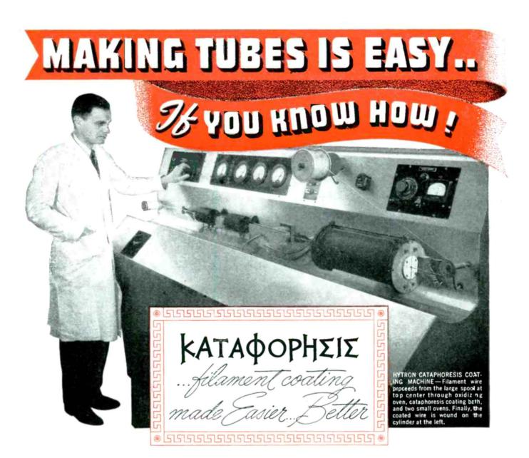
A jawbreaker from the Greek, cataphoresis means simply "the movement of suspended particles through a fluid under the action of an applied electromotive force." At Hytron, filaments are not *sprayed* with electron-emissive coating, because that way precise control cannot be achieved. Rather, coating is electrically deposited by the cataphoretic movement of the carbonate molecules.
