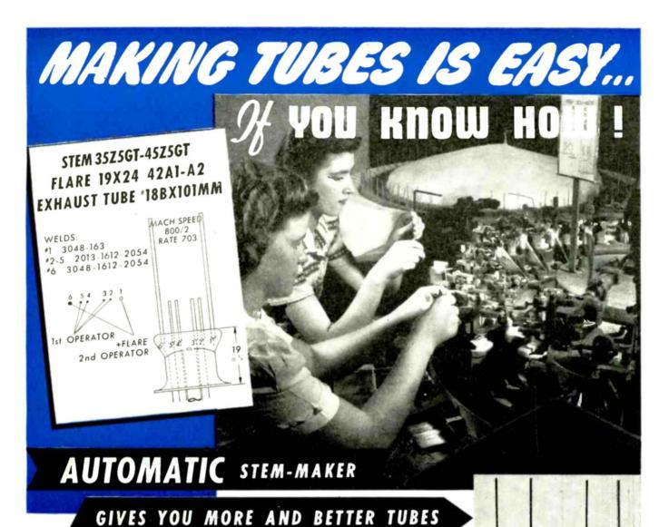
Making a radio tube stem is apparently easy. By gas flames, one merely seals stem wires and exhaust tube into a glass flare. High-speed production, however, raises problems of know-how. Expert adjustment of temperatures and timing is vital. To give you trouble-free performance, there must be absence of glass malformation, strains, cracks—air-tight wire seals—strict adherence to dimensions.
