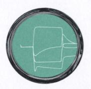
a Storage Tube designed for the display and retention of electronic signal traces. The retention feature of the Memotron Tube allows a number of signals to be superimposed or stacked vertically for comparison. The tube is used extensively in image-retention oscilloscopes such as the Hughes Memo-scope ® unit.
