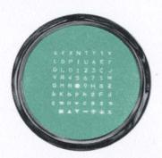
a Hughes Cathode Ray Tube for displaying a matrix of letters, numerals, symbols. There are 63 characters available in standard or special alphabets. With a 21 inch tube as many as 4500 characters can be displayed on the tube face. The Typotron Tube has the ability to retain the character display for extended periods, making it especially useful for air traffic control and as a visual readout with computers.
