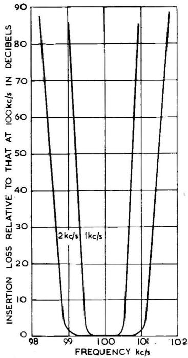
Fig. 4. Filter response (HR.91)
