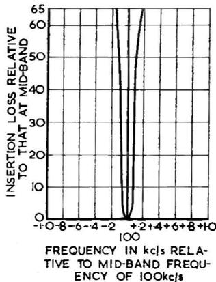
Fig. 10. Carrier filter response (HR.93)
