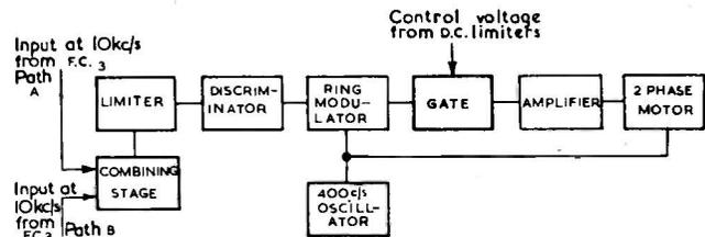
Fig. 15. Automatic frequency control (HR.11)
