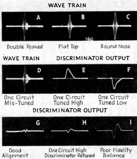
Fig. 1—Oscilloscope wave trains and output of discriminator for various conditions of tuning
