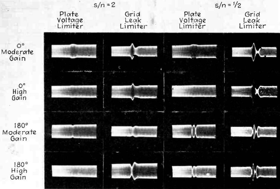
Fig. 4—(above) Oscillograms demonstrating the relative effectiveness of plate voltage and grid leak limiters . . . Fig. 5—(below) Oscillograms of noise and discriminator output with carrier tuned to edge of the pass band
