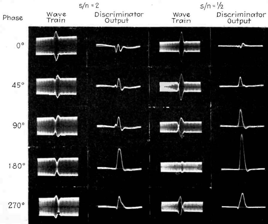
rier wave are added with various phase angles. The second column illustrates the output of the discriminator for the same conditions. It can be seen that the zero and 180-degree phase angles produce the maximum amount of amplitude modulation and the minimum output from the discriminator. The 90-degree and 270-degree phase angles produce minimum amplitude modulation and maximum output from the discriminator. The intermediate phase angles produce both types of modulation.
