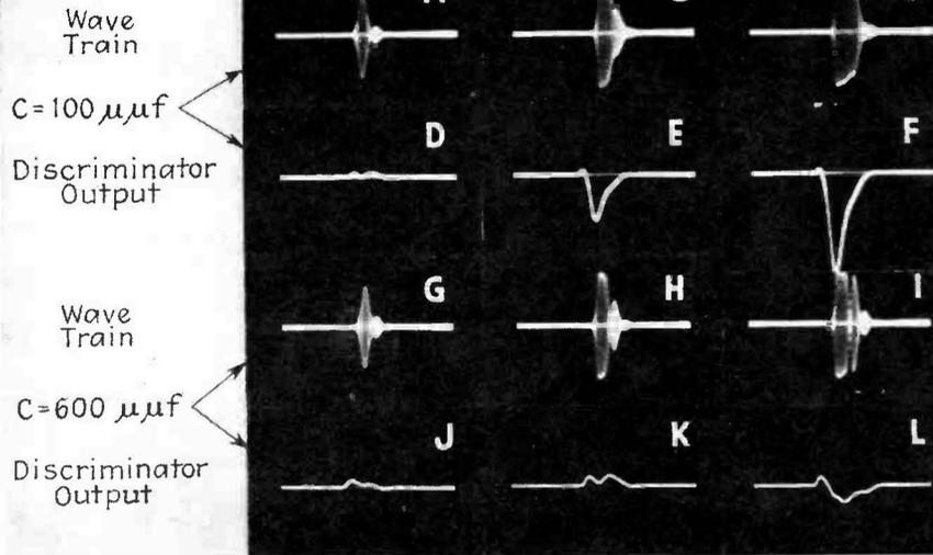
Fig. 2—Oscilloscope wave trains and output of discriminator showing detuning due to grid current at higher amplitudes
