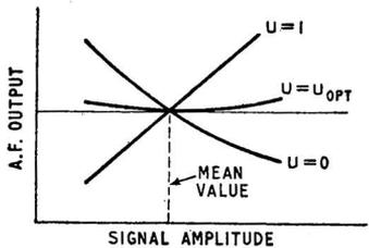
Fig. 11. Showing variation of a.f. output with input signal amplitude for a fixed frequency input signal ( $\Delta f$  small).
