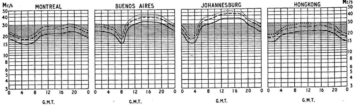
THE full curves given here indicate the highest frequencies likely to be usable at any time of the day or night for reliable communications over four long-distance paths from this country during May.
