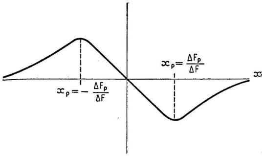
Fig. 12. Showing variations of output ( $y = E/E_s$ ) against input signal frequency ( $x = \Delta f/\Delta F$ ).
