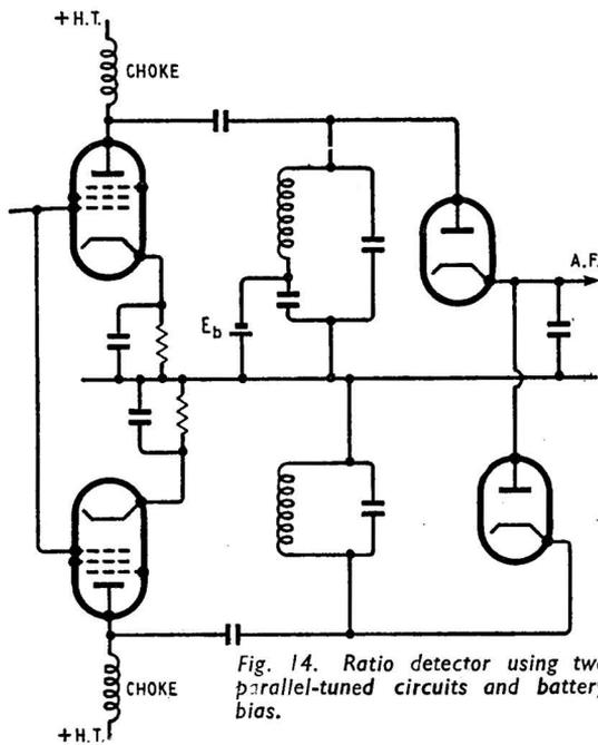
Fig. 14. Ratio detector using two parallel-tuned circuits and battery bias.
