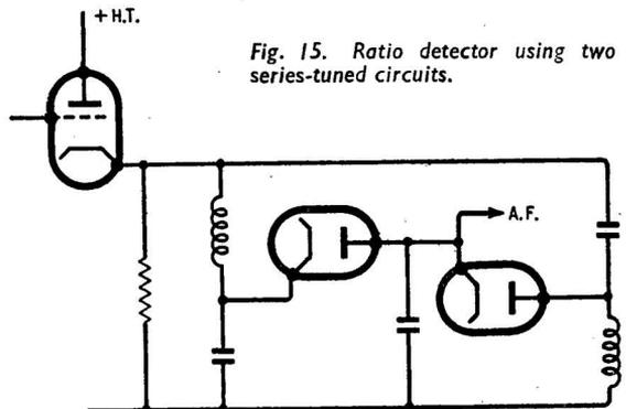
Fig. 15. Ratio detector using two series-tuned circuits.
