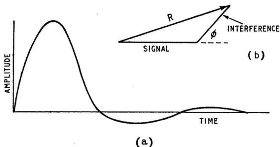
Fig. 7. (a) Waveform of i.f. output due to a pulse of interference and (b) vector relationship of signal and interference.
