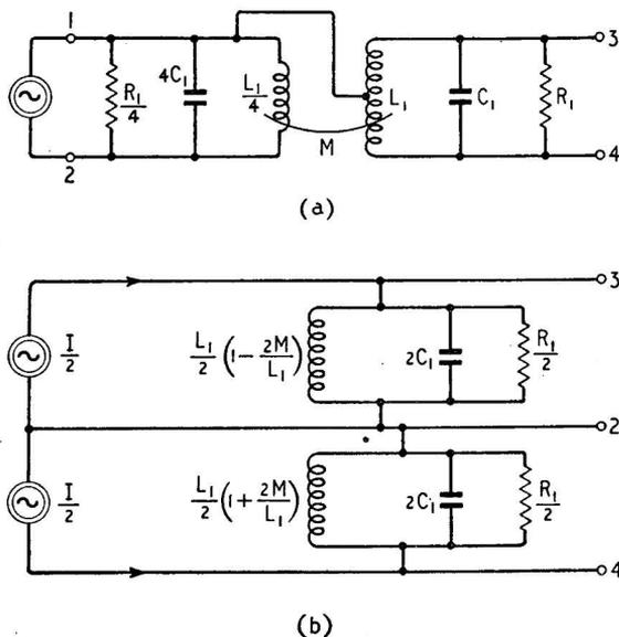
Fig. 13. Identical performances are given by these forms of (a) the Foster-Seeley and (b) the Round-Travis circuits
