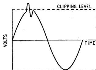
Fig. 11. When the interference pulse coincides with a peak of modulation, clipping may remove part of the pulse and increase noise.
