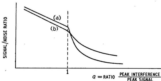
Fig. 9. Signal/noise ratio with impulsive interference for (a) wide-band and (b) narrow-band discriminators.
