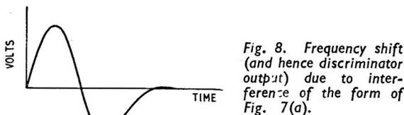
Fig. 8. Frequency shift (and hence discriminator output) due to interference of the form of Fig. 7(a).
