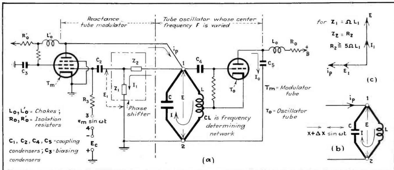
Fig. 1—Schematic wiring diagram of reactance tube modulator and associated oscillator tube. The assigned carrier frequency is  $F = \Omega/6.28$ ; the modulating frequency is  $f = \omega/6.28$
