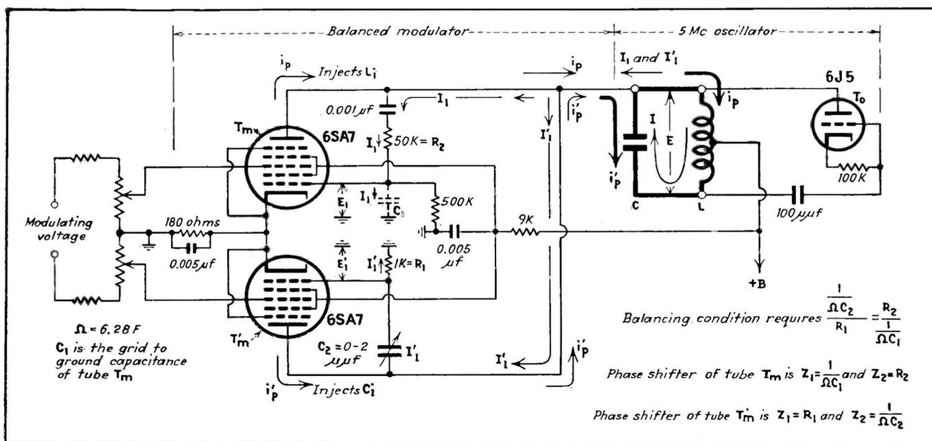
Fig. 4—Diagram of balanced modulator and oscillator tube to illustrate the current and voltage conditions which occur for a balanced modulator
