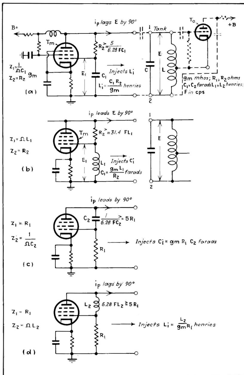
Fig. 2—Schematic wiring diagram of four types of reactance tube networks, with their design equations
