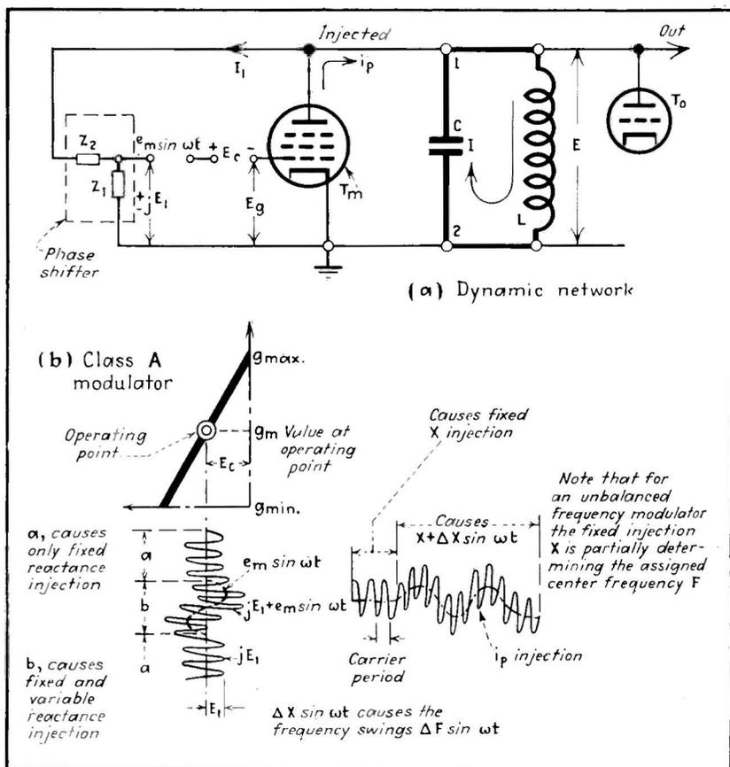
Fig. 3—Dynamic network of oscillator tube and reactance tube injector circuit (a), with wave forms of modulated and unmodulated signals illustrating variation of transconductance of modulator tube
