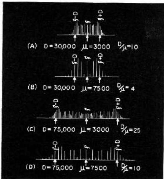
Fig. 3—Spectrum distribution in frequency-modulated system, for various deviation frequencies,  $D$ , and modulating frequencies,  $\mu$ . Compare top and bottom curves for which  $D/\mu = 10$  in both cases
