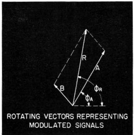
Fig. 4—Rotating vectors representing f-m signals. Vector  $B$  is the interfering signal,  $A$  is the desired signal,  $R$  is the resultant
