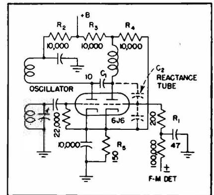
FIG. 6—A tuned-grid oscillator and afc reactance-tube circuit
