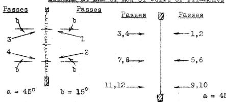
Note: Where filaments are observed to be insufficiently coated at certain points or sections, a shot or pass may be made at these points or sections to bring coating to desired thickness. Each of the above diagrams represents the passes in 1 covering. To bring coating diameter to specified limits, more than one coating may be required.
