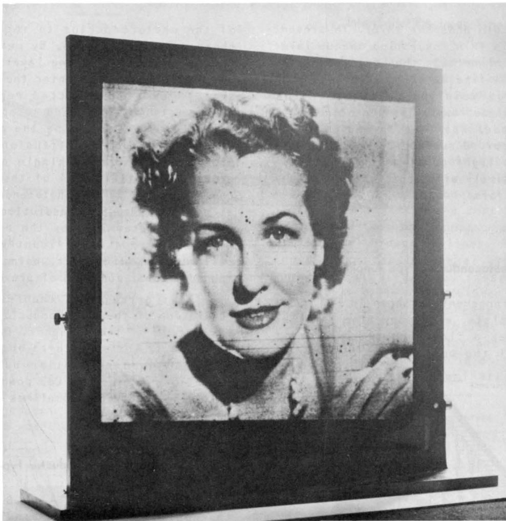
Fig. 7 - Photograph of grooved type light amplifier showing amplified picture resulting from a projected image.
