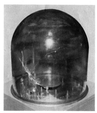
A bell jar with an eight-inch crack was coated with RCA plastic No.33-L-614 in the approved manner and evacuated to less than 50 microns pressure. While under vacuum, the jar was subjected to an impact force of 175 pounds, applied by means of an iron-ball pendulum. This force caused the jar to shatter, but none of the broken glass was sucked into the pump line, nor did any glass break free from the plastic.
