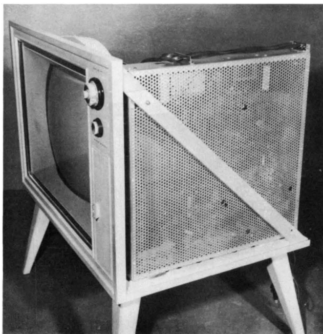
Fig. 6 - The bottom of the chassis and the rear of the cabinet are shielded to reduce radiation.
