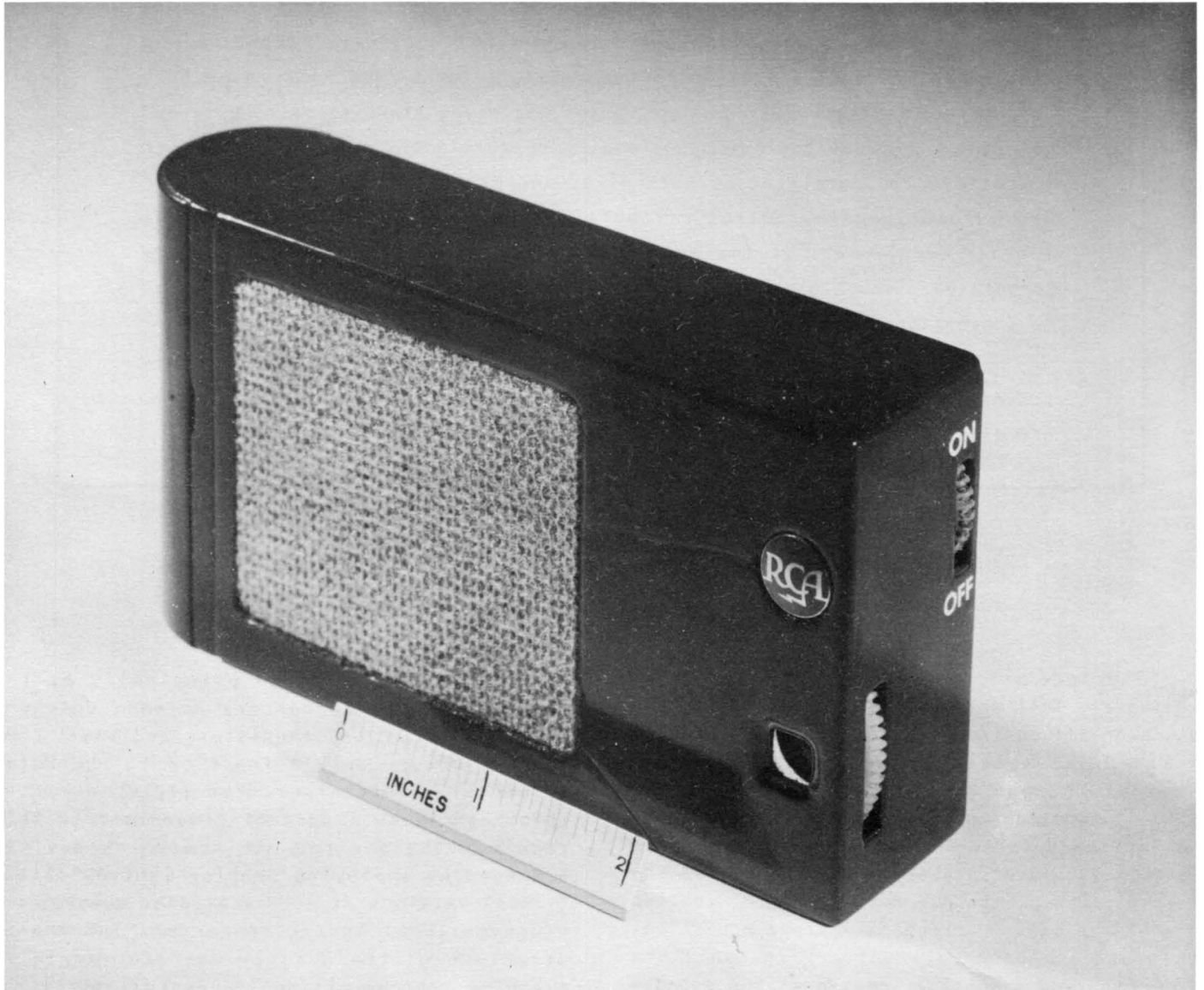
Fig. 1 - Developmental pocket-size broadcast receiver.
