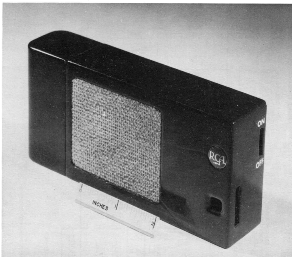
Fig. 2 - Receiver case with alternative battery case attached.
