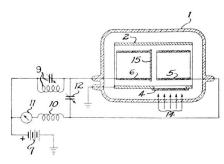
tiplier, external circuit means for operating the other of said structures as an electron multiplier oscillator, and means for connecting the oscillator output to energize said multiplier.
