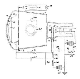
ment thereof, an electron gun for bombarding said picture area with a beam of electrons, and a conductive electron collector adapted to be impinged by said beam of electrons extending in an area parallel to said picture area and spaced adjacent thereto, said collector having a concave curvature in the direction of said beam of electrons substantially equal to the curvature of said picture area.
