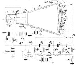
gized to unidirectional potentials increasing in accordance with the intensity of said beam and the position of said beam.
