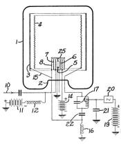
1. A signal translating device comprising means for producing a primary flow of electrons, means for modulating the intensity of said electron flow in accordance with an input signal, means for multiplying said modulated electron flow by secondary emission, means for utilizing said multiplied electron flow to generate electrical oscillations, means for controlling said primary electron
