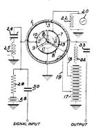
1. The method of signal amplification which comprises the steps of causing the initiation of a space flow of electrons, causing said flow to be subjected to alternate processes of attenuation by electron absorption and multiplication by secondary emission, and applying the signal to vary one of said processes.
