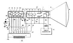
cluding a plurality of secondary emissive multiplying stages, an electron source for supplying electrons to the first of said multiplying stages, means for controlling the flow of electrons through said multiplier in accordance with an input signal, and means for coupling the output of said multiplier to said pair of deflectors, thereby to obtain an indication representative of said input signal and of its average value.
