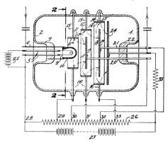
1. An electron multiplier comprising a series of alternately cylindrical and plane secondary electron-emitting surfaces mounted in cascade, each of said cylindrical surfaces and each of said plane surfaces being progressively increased in size from one end to the other in the series, and means for liberating secondaries from the smallest surface.
