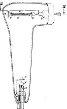
1. Means for producing a visual image comprising an envelope containing means for producing a cathode ray beam, an open mesh fabric screen, means for directing said beam over successive elemental areas of said screen to produce an incandescent image thereon by the impact of electrons intercepted thereby, and transparent means for returning beam electrons to said screen that pass therethrough, said transparent means being positioned between said screen and an observer viewing said screen.
