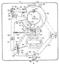
5. In an automatic phonograph having a turntable and a movable pickup arm for cooperating with a record on said turntable; initiating apparatus comprising a driving means rotatable with said turntable; coupling means slidably connected with said pickup arm and being movable thereby a predetermined distance in a first direction
