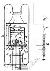
1. An electron multiplier, comprising an evacuated envelope having therein an electron source, a plurality of secondarily emissive multiplying stages, an electron-permeable screen surrounding said multiplying stages and forming to a Faraday cage, the last of said stages being completely non-permeable to electrons emitted from the next previous stage and being completely permeable to secondary electrons emitted by said last stage, and means for withdrawing electrons from said last stage.
