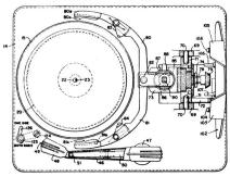
5. In an automatic phonograph having a rotatable turntable for supporting a stack of records of different diameters, a pickup arm for reproducing the top record on said turntable, and a record magazine; the combination of means
