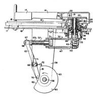
ber for elevating said pickup arm, rotatable hydraulic means for operating said rotatable member and swinging said pickup arm horizontally beyond the record on said turntable and returning said pickup arm into engagement with the initial groove of said record on said turntable, and operating means for controlling said hydraulic means.
