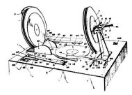
1. In an automatic phonograph including a turntable, a pair of arms disposed in movable relation with respect to a record on said turntable, record-engaging means at the ends of said arms adjacent said record comprising a pair of rotat-
