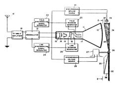
1. In a color television signal receiving system, means for reproducing a television image in a plurality of separately and intermittently produced different colors, and means for producing intermittent light impulses of said different colors in alternation with the production of said image colors.
