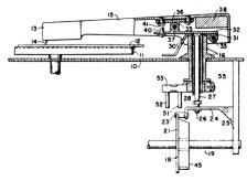
1. An automatic record-changer apparatus comprising a turntable, a pickup arm for cooperating with a record on said turntable, a movable cam means for moving said pickup arm, and a means operatively associated with said cam means and said pickup arm and movable by said cam means for imparting to said pickup arm a relatively fast outward movement and a relatively slow inward movement.
