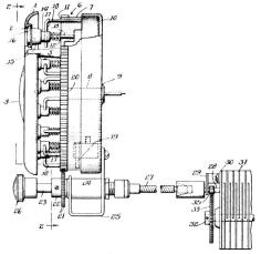
shaft for rotating said condenser to tune said receiver to any other desired broadcast station.
