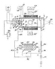
stresses set up when energized to a predetermined steady collection potential, an oscillator connected to said electrode, and circuits maintaining the frequency of said oscillator substantially higher than the natural period of said collecting electrode.
