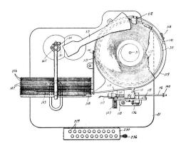
in sequence, automatic means for rotating said magazine to reverse the records and present opposite sides thereof to said transfer means and manually actuated selective means movable into the path of movement of the magazine effective to arrest the movement thereof and render ineffective the automatic progressive positioning thereof in sequence, to present the selected side of a selected record for transfer to said turntable.
