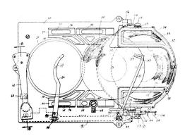
horizontally disposed, means for swinging said magazine from one horizontal position to the other after each record is reproduced, and means for displacing said magazine vertically relative to the turntable and transfer means during every alternate swinging movement so as to receive a record below the group when in uppermost position and above the group when in lowermost position.
