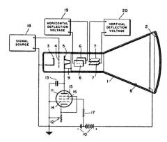
coating of current derived from said source of energy, and electronic means for varying the magnitude of the current flow, whereby to vary the potential impressed upon said anode.
