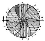
A composite filter disk structure comprising a hub and a plurality of sectorially shaped elements, the radially extending edges of which are of arcuate form and shaped to engage each other in tongue and groove fashion, each of said elements being secured to said hub and being transparent to light of a particular color.
