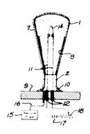
2. The method of temporarily covering the inner wall of an envelope having a narrow opening with a resilient sheet during the evaporation of metal therein which comprises rolling said sheet upon itself until the roll is of small enough diameter to enter the opening, releasing the roll to expand said sheet to form a band covering an area of said wall, evaporating metal within said envelope, re-rolling said sheet and removing it while rolled through said opening.
