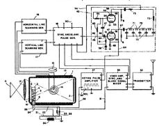
20. The method of transmitting and receiving television pictures in relief comprising the steps of deriving successive groups of picture signals representative of an object to be transmitted, transmitting said groups of picture signals, receiving said groups of picture signals, receiving said successive groups of picture signals to obtain successive complete television images, and periodically displacing one of said television images with respect to another one of said television images.
