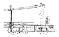
1. In a record changer assembly including a turntable, a support for records above the turntable, means operatively associated with said support and including a rotatable pinion for discharging the records singly from said support onto said turntable, a tone arm adapted to be raised and lowered and to be reciprocated over the turntable, means for actuating said tone arm
