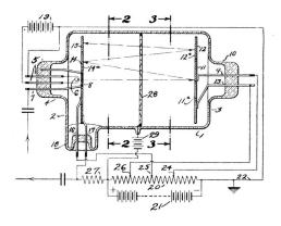
spaced groups of concentrically spaced elements, each group being in the same plane.
