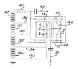
each apertured electrode, said tubular cathode, secondary emissive cathodes and apertured electrodes being energized in the order recited to increasingly higher potentials, and means for liberating primary electrons along the axis of said tubular cathode.
