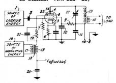
1. In a modulation circuit, an electron discharge device having at least a control grid, a suppressor grid and an output electrode, means for applying carrier energy to said control grid,
