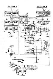
1. In signalling apparatus, in combination, two signal receivers, means for comparing the relative strengths of the two signals received and for producing a potential the polarity of which
