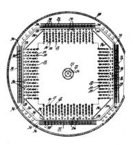
and said target to produce secondary electrons responsive to electrons from said source, each of said plurality of electron multiplying means being positioned in said tube to provide electrons to a different area of said target, and bias means connected to each of said electron multiplying means to control the flow of said secondary electrons to selected areas of said storage target.
