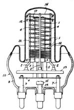
1. A control electrode for electrical discharge devices comprising a wire helically wound on a plurality of substantially parallel posts, each post comprising two cooperating clamping members having transverse grooves on their adjacent faces which coact to grip the respective turns of said wire, and a helical binder closely surrounding each said post.
