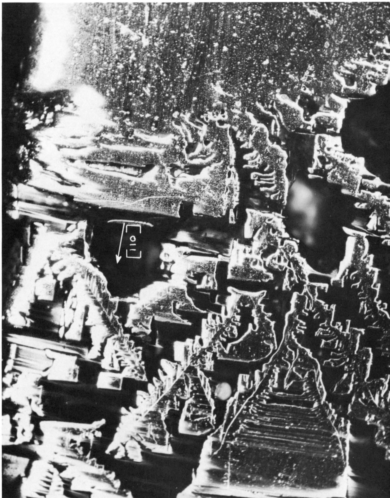
Fig. 10 - Cross section of a recrystallized region in the 100 plane. The parent crystal is at the top. Note the thick overgrowth region in the 110 direction (arrow), and at the lower right hand corner the stack of 111 facets appearing in cross section.
