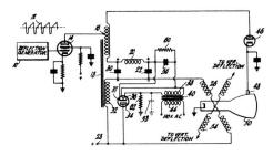
1. In an electrical circuit, the combination of, a reference potential datum, a discharge tube having at least an anode, cathode and heater electrode, said tube having a predetermined maximum heater-cathode voltage rating, an output terminal at which appears a signal waveform relative to said datum having a peak voltage in excess of said heater-cathode voltage rating, a set of heater power supply terminals coupled with said heater for excitation thereof,
