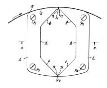
tapered inwardly in the direction of said gap and terminating adjacent to said gap in projections of substantially uniform cross-section, said magnetic structure being of stacked laminated construction each lamina of which being of duplicate size and shape.
