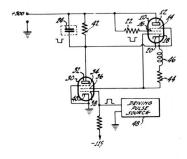
2. A system for driving a capacitive load comprising a first tube having anode, cathode and control grid electrodes, a second tube having anode, cathode, control grid and screen grid electrodes, said first tube cathode being connected to said second tube anode, said capacitive load being connected across one of said tubes, means to apply potentials to said first and second tubes to maintain said first tube conductive and said
