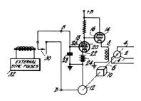
lationship between said two groups of pulses, and a means for utilizing said control voltage to vary the current in said winding in such manner as to maintain the phase between the two groups of pulses at a constant value.
