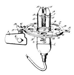
acoustic resistance therefor and including a supporting device, and flexible means connecting said motor assembly to said supporting device thereby to flexibly support said motor assembly from said supporting device.
