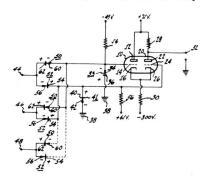
larity connected between said signal input terminals and said first tube grid, means to pass signals of only the opposite polarity connected between said signal input terminals and said second tube grid and means to derive an output from said second tube anode when the signals existing simultaneously on said first and second tube grids have the same amplitude.
