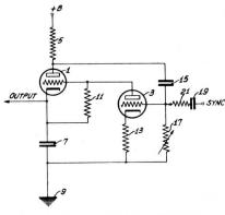
A saw-tooth wave generator comprising in combination, first and second electron discharge devices, each of said devices having a cathode,
