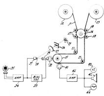
1. A sound recording system comprising means for simultaneously recording a photographic record and a magnetic record on the same film of the same sound waves, and means for simultaneously reproducing said magnetic record for monitoring said photographic record.
