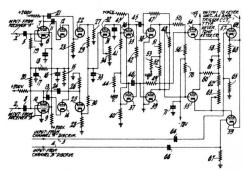
1. In a gating circuit, a pair of electronic valves each having at least anode, cathode and grid electrodes, means for applying a pair of signals to be gated each to a respective grid electrode,
