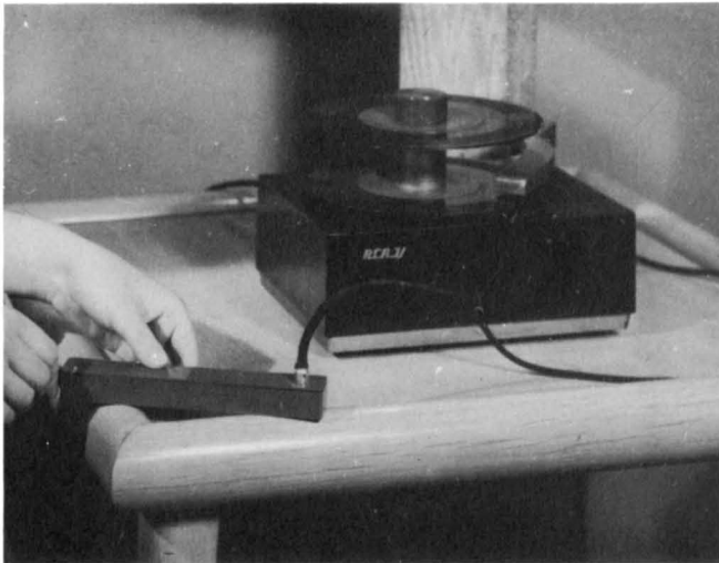
Fig. 42 - Transistor oscillator unit attached to record player.
