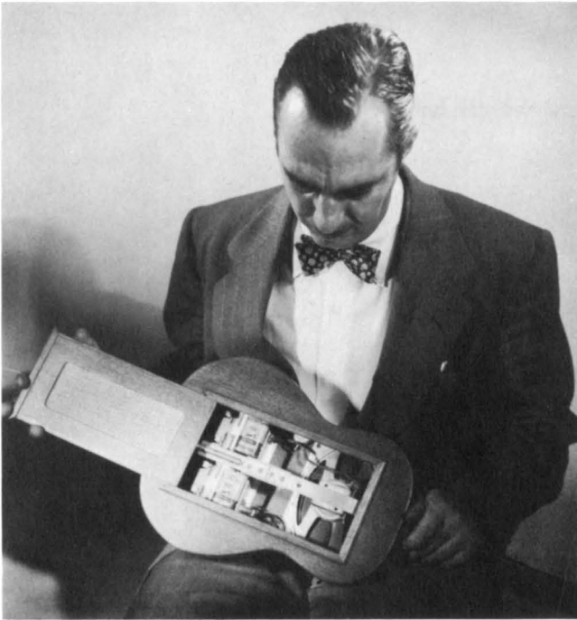
Fig. 56 - Back view of ukelele showing transistor amplifier and speaker housed within the body of the instrument.
