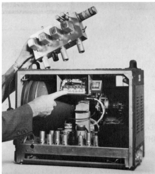
Fig. 33 - Industrial television transistor sync generator chassis compared with its all-tube counterpart.
