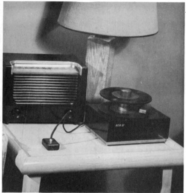
Fig. 38 - Transistor phono-jack connected to record player, transmitting signal to receiver.
