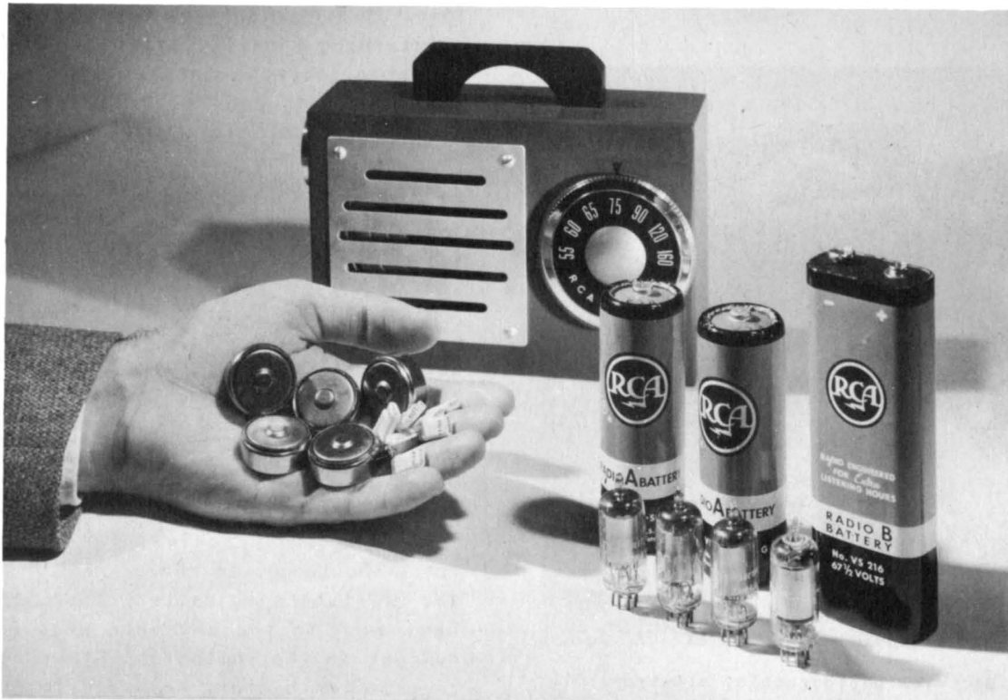
Fig. 20 - All-transistor portable receiver. Its batteries and transistors are compared with the tubes and batteries which would be required in an all-tube receiver of similar performance.
