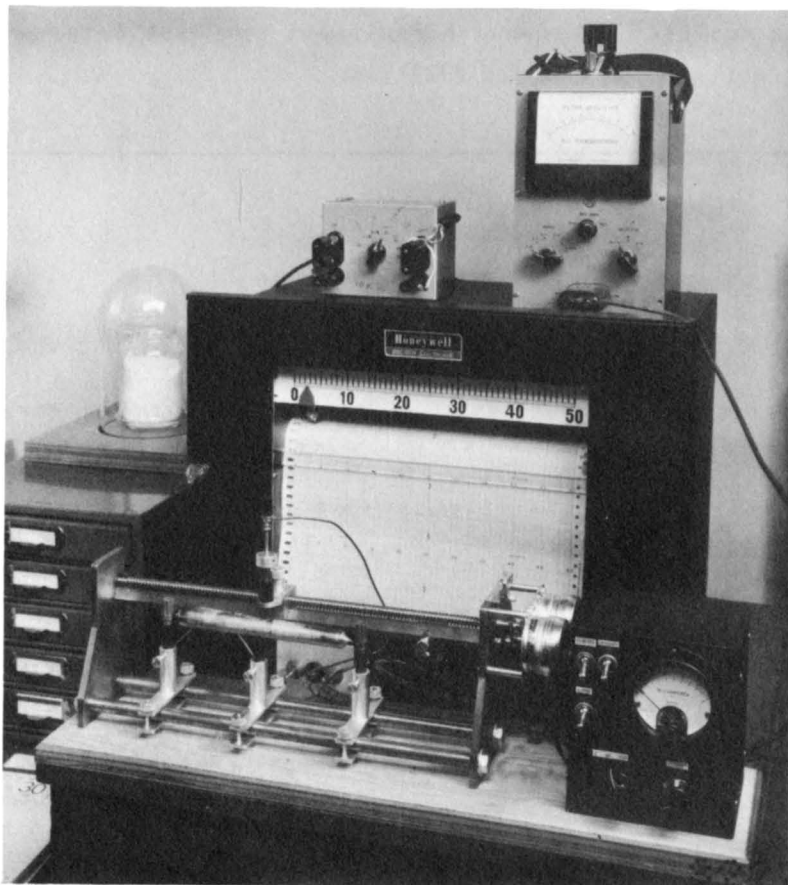
Fig. 1 - Equipment used in resistivity measurements.
