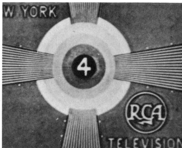
Fig. 5 - Photograph of test pattern, interlaced, without spot wobble.
