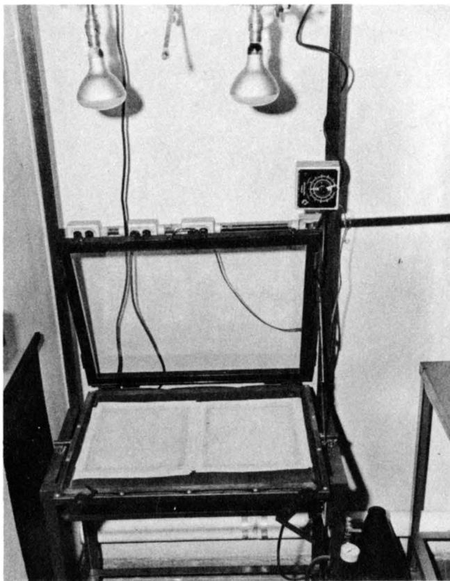
Fig. 9 - Vacuum frame and light for making gelatin stencil. Frame open.
