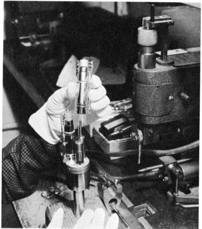
Fig. 26- Assembly of mount on mandrel.
