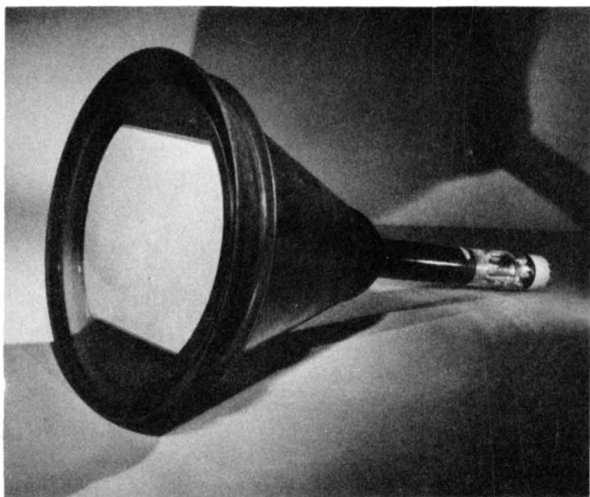
Fig. 1 - Photograph of an RCA three-gun tri-color kinescope.
