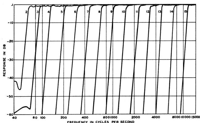
Fig. 7 - The response frequency characteristics of the fourteen high pass filters used in the nonlinear distortion analyzer.
