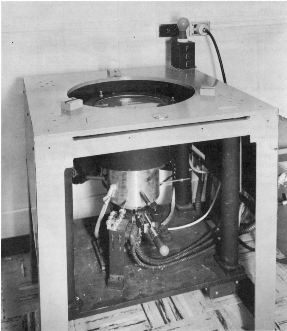
Fig. 20 – Modified optical lighthouse showing placement of radial correction lens.
