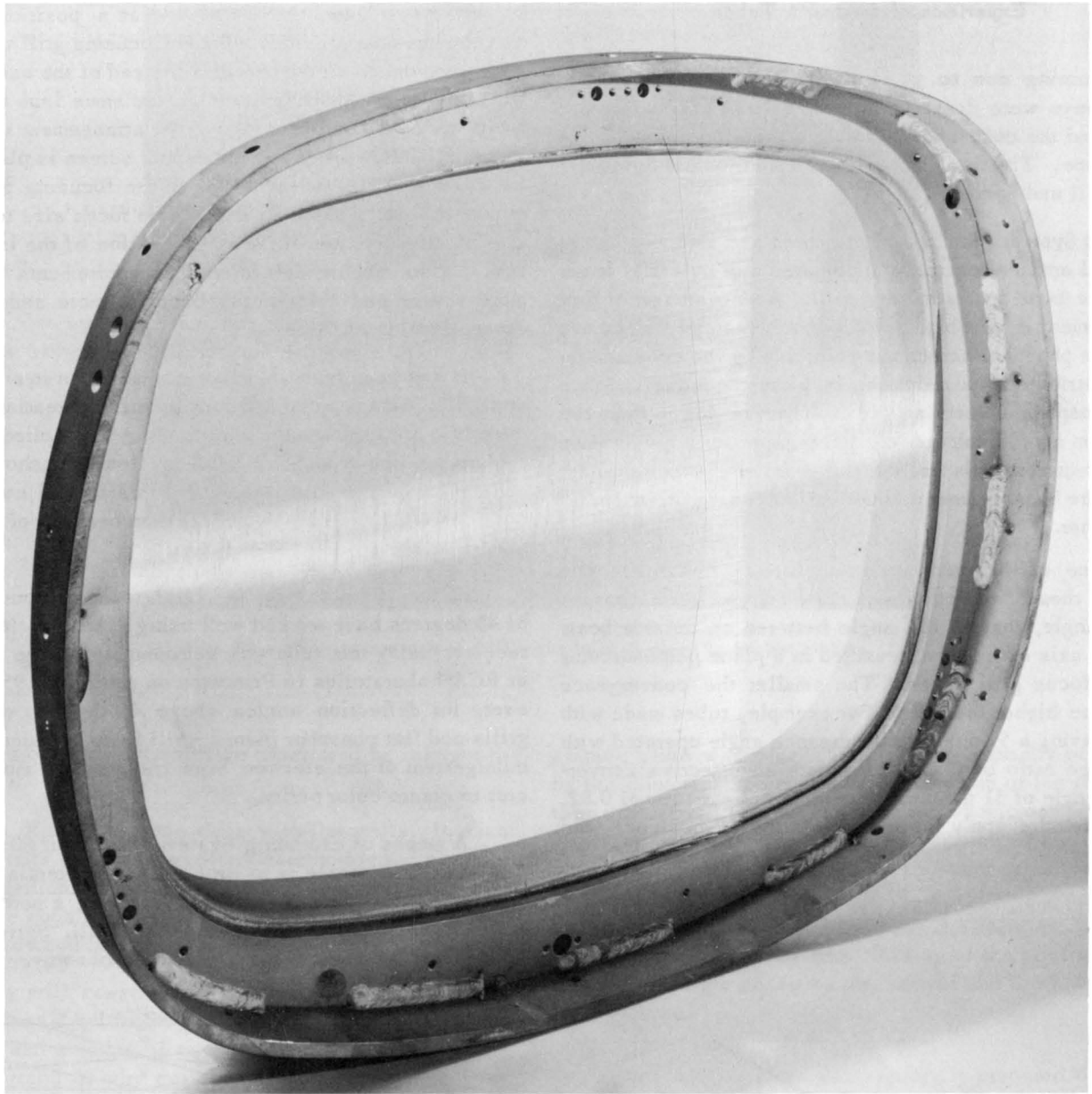
Fig. 19 – Focusing and auxiliary grill structure for a 24 inch rectangular tube.
