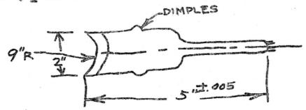
Neck Down: They are in the habit of putting a constriction in the neck of high voltage tubes to give a convenient place to attach snubbers and reduce stray emission from the lower neck.
