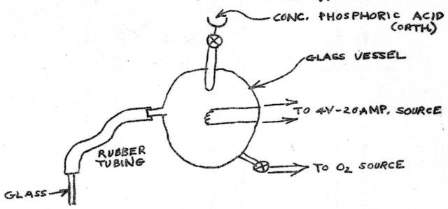
The acid is dropped, drop by drop onto the hot filament, causing a dense cloud of smoke. A see whiff of O2 is introduced and blows the smoke into a clean bulb through the hosing and glass tube. The bulb at this point looks as if someone had puffed cigarette smoke into it. The smoke is left stand 1 minute. A
