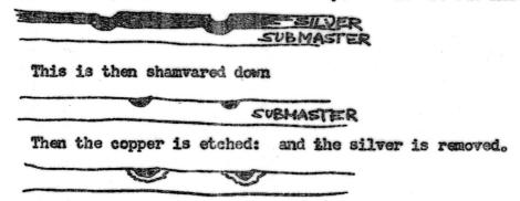
All very easy for people who make phonograph masters. This mesh is most painstakingly examined uner a microscope and sections that cannot be used (filled holes etc.) are rejected.
