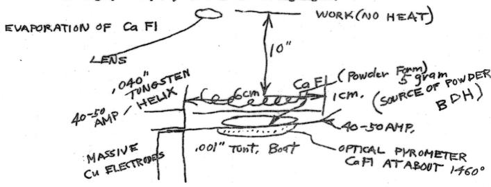
The set up is as I have illustrated in the genuine sketch I drew all by myself (God). A little double convex lens of any sort is mounted adjacent to and with its plane aligned with the plane of the work. The work is very slowly brought up to temperature (about 45 min.). The little lens is only used to watch
