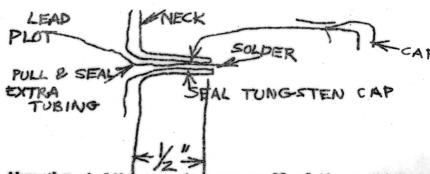
Leads are brought throughneck like so. As many as 32 of these stick out a single neck. The leads are button hooked out before the tungsten cap is sealed on with a sort of housekeeper deal. All hand torch work!
