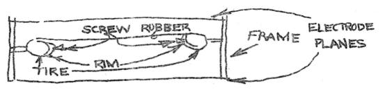
This device seems to work fine. Four upright posts support the wheel and two datum planes from which electrodes poke up or down. Since in multiplier tubes, they always assume negligible initial velocity, no ramp is employed. A 1/8" ball is brought to rest through a piece of tubing and is released by raising the end of the tubing. No recording apparatus is used to trace the path.
