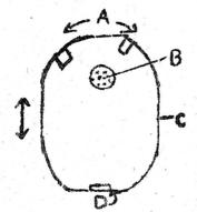
Fig 2 shows a top section. The two fires A are moved up to the rotating neck B for approximately 8-10 seconds. Then, the supporting ring C is moved in the direction shown until the water cooled edge D comes in contact with the neck.
