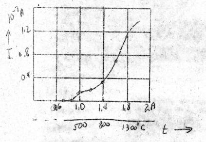
Dependence of the emission current I on the filament current i of a .15 mm. filament. The bottom scale gives the temperature in degrees centigrade.
