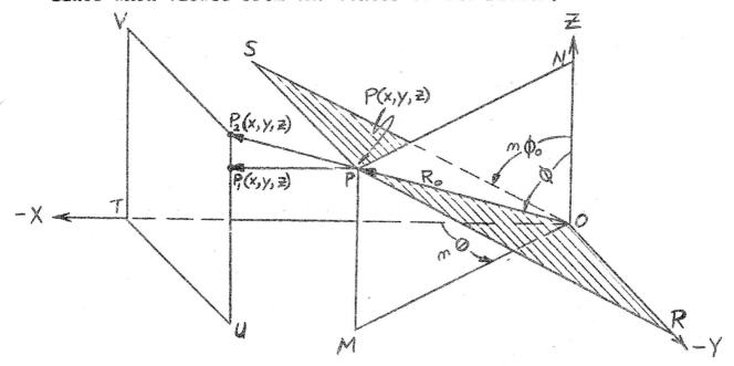
In Figure 1, the plane MN is representative of the family of planes which define constant projected angles (integral multiples of  $\theta_0$ ) in the horizontal plane XY. The plane RS represents the family of planes defining constant projected angles (integral multiples of  $\theta_0$ ) in the vertical plane XZ. The intersections of the families of MN and RS with a sphere of radius OP are the desired loci of the lenticle centers.
