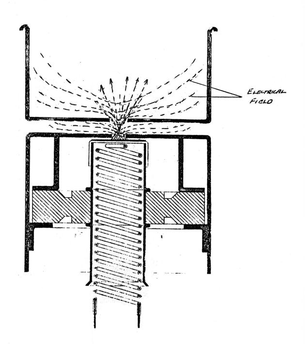
are not in line, the field could be of elliptical shape and the resultant projection of this shape can be readily seen at test. The picture quality is dependent on the beam shape being round and of proper size.
