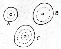
The screen grid tube - C - might be considered as a three element tube - A - where the plate is in place of the screen grid and the plate voltage is computed as the effective voltage in - another - three element tube - B - where the screen grid took the place of the control grid\*
