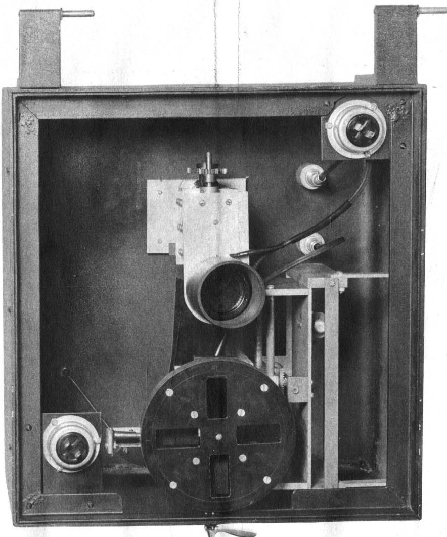
1022 342 G-E LIGHT AND COLOR MEASUREMENT EQUIPMENT FOR CATHODE-RAY TUBE. REAR VIEW.
