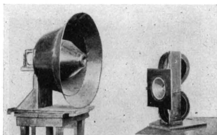
FIG. 30.—MOVING COIL TYPE LOUD SPEAKER UNIT WITH PERMANENT MAGNET FIELD AND THREE-PASS EXPONENTIAL HORN
