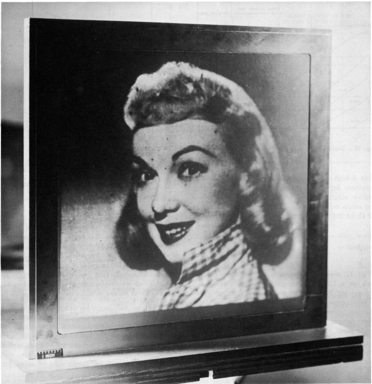
Fig. 12 - Photograph of the output picture produced on a 12" light amplifier with a low-level image projected from behind.
