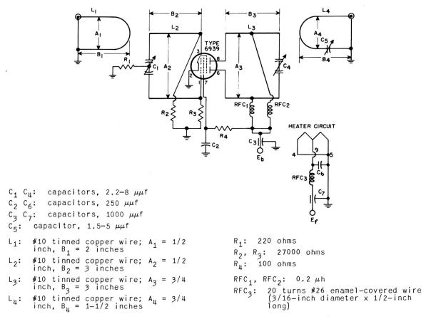
Fig. 1 - 500-megacycle push-pull rf power-amplifier circuit using the 6939.
