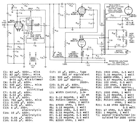
Fig. 1 - Horizontal-Deflection and High-Voltage Circuit.
