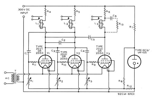
R1 R2 R3: Timing control, potentiometer, 5 megohms
