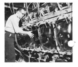
drying rods and an air manifold is mounted on tracks under the conveyor and is synchronized to travel with it. The rods are raised into the bulbs and about 100 cu ft per hour of heated, filtered air is forced into the bulb to dry the screen coating. These rods have especially designed tips that provide proper air currents, pattern, and volume.
