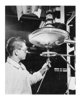
The operator places the bulb face against a live vacuum chuck in the burrotating machine and marks the propaint dimensions on the neck using a special gage. The special knee-action type paint applicator is then inserted into the rotating bulb and, by skillful use of the applicator controls, a uniform coating is applied to the cone and neck. After drying the inside paint, the bulbs are transported by overhead conveyor to the baking station.
