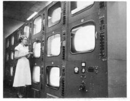
Statistical quality control inspection and test stations between final test and packing help maintain the quality level required in this highly competitive field. In addition, the product is life tested on expensive, carefully maintained equipment to assure shipment of products consistent with General Electric Company's high quality standards.
