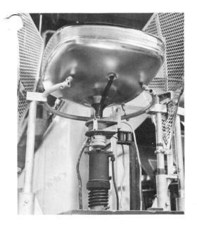
After evacuation of all gases, it is necessary to seal or "tip-off" the exhaust tubulation projecting from the stem seal. By trade definition, a bulb becomes a tube when it has been exhausted and tipped. Originally, this was a hand operation, but automatic tipping machines have replaced the method and provide more uniform processing. These are small electrical radiant tipping ovens that supply a controlled localized source of heat, resulting in an improved tip and simplification of the process.
