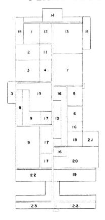
I RECEIVING WHSE. 2 WASH AREA 3 SCREEN AREA 4 FILM AREA 5 INSIDE PAINT, INSP. 6 ALUMINIZE 7 BAKEOUT 8 GUNSEAL 9 EXHAUST, G.F., BASE IO SPARK, AGE, TEST II OUTSIDE PAINT, INSP. 12 PACK AREA 13 P.A., STORAGE AREA 14 TRUCK WELL 15 TRAIN WELL 16 SALVAGE AREA 17 PARTS, MOUNTS 18 TOOL ROOM 19 18M OFFICE, DEV. AREA 20 ISM MANUF, AREA 21 18 M WAREHOUSE 22 FACILITIES AREA 23 C.R.T. GEN. OFFICES
