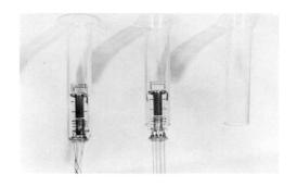
The electron gun mount consists of two major parts — the electron gun and the stem. The gun is that portion of th tube supplying the electron beam that activates the screen to produce the television picture. The stem is used for supporting and supplying voltage to the gun.
