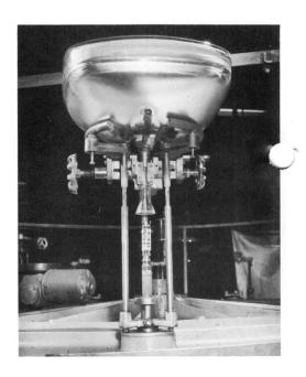
is unloaded from the machine in the final position. The overhead conveyor delivers the bulb to the next process.
